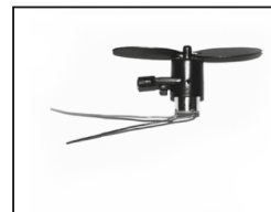
Motor (forward/backward flight)
