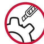
**EN** Burrs on the jumper should be gently grinded with the sandpaper or carefully cut with the stationery knife.
