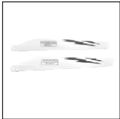
Upper main rotor blades (A) XBM13-07
